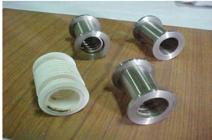
FIG. 25. Mechanical gadgets. (In clockwise direction from left bottom: bellows, spool piece with helical coil, threaded spool piece with 3 mm pitch, and threaded spool piece with 7 mm pitch).
